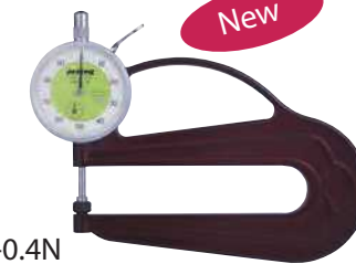
H-0.4N Graduation: 0.01mm Range: 0~10mm Measuring force initial pressure 0.4N
