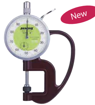
G-0.4N Graduation: 0.01mm Range: 0~10mm Measuring force initial pressure 0.4N
