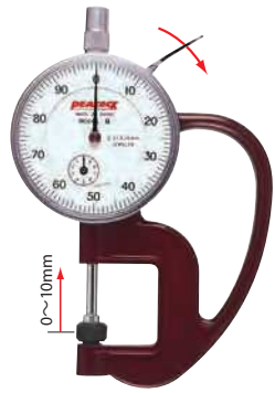
G Graduation: 0.01mm Range: 0~10mm φ 10mm flat contact point and anvil (Ceramic)
