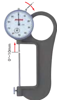
G-4 Graduation: 0.01mm Range: 65mm Spherical contact point Anvil side is adjustable More than 10mm range is comparative measurement.
