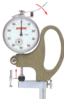
G-3 Graduation: 0.01mm Range: 30mm φ 10mm flat contact point and anvil (Ceramic) Anvil side is adjustable More than 10mm range is comparative measurement.
